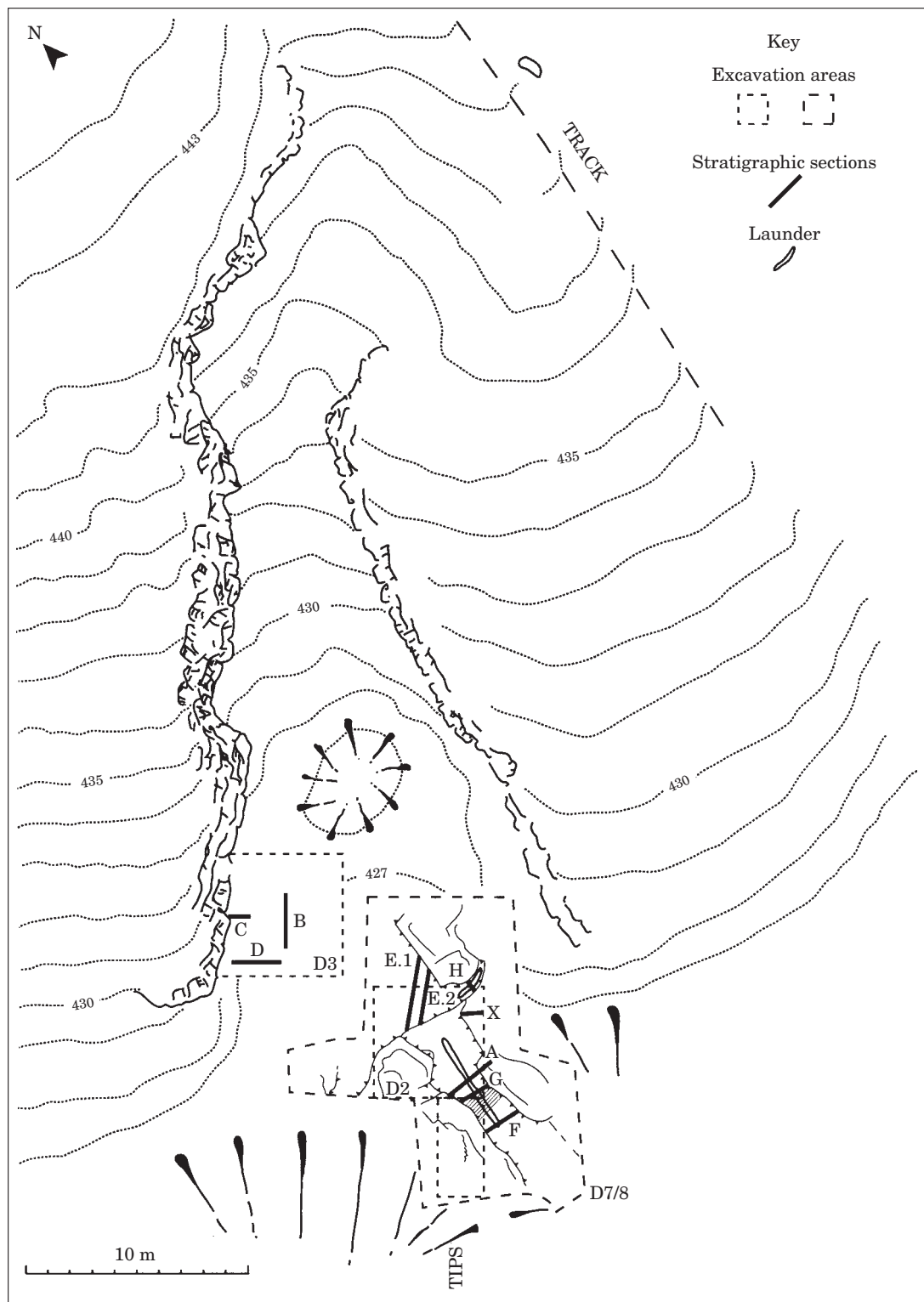
Figure 2. Plan of the Bronze Age mine showing the position of the stratigraphic sections.
